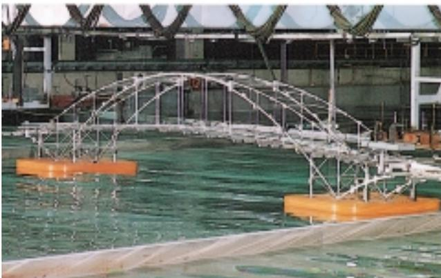
Photo 4 Elastic Model Experiment on In-wave Elastic Response
