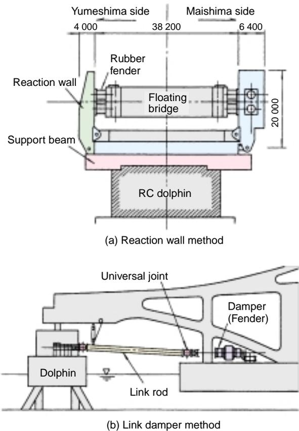
Fig. 6 Schematic of Mooring Systems
