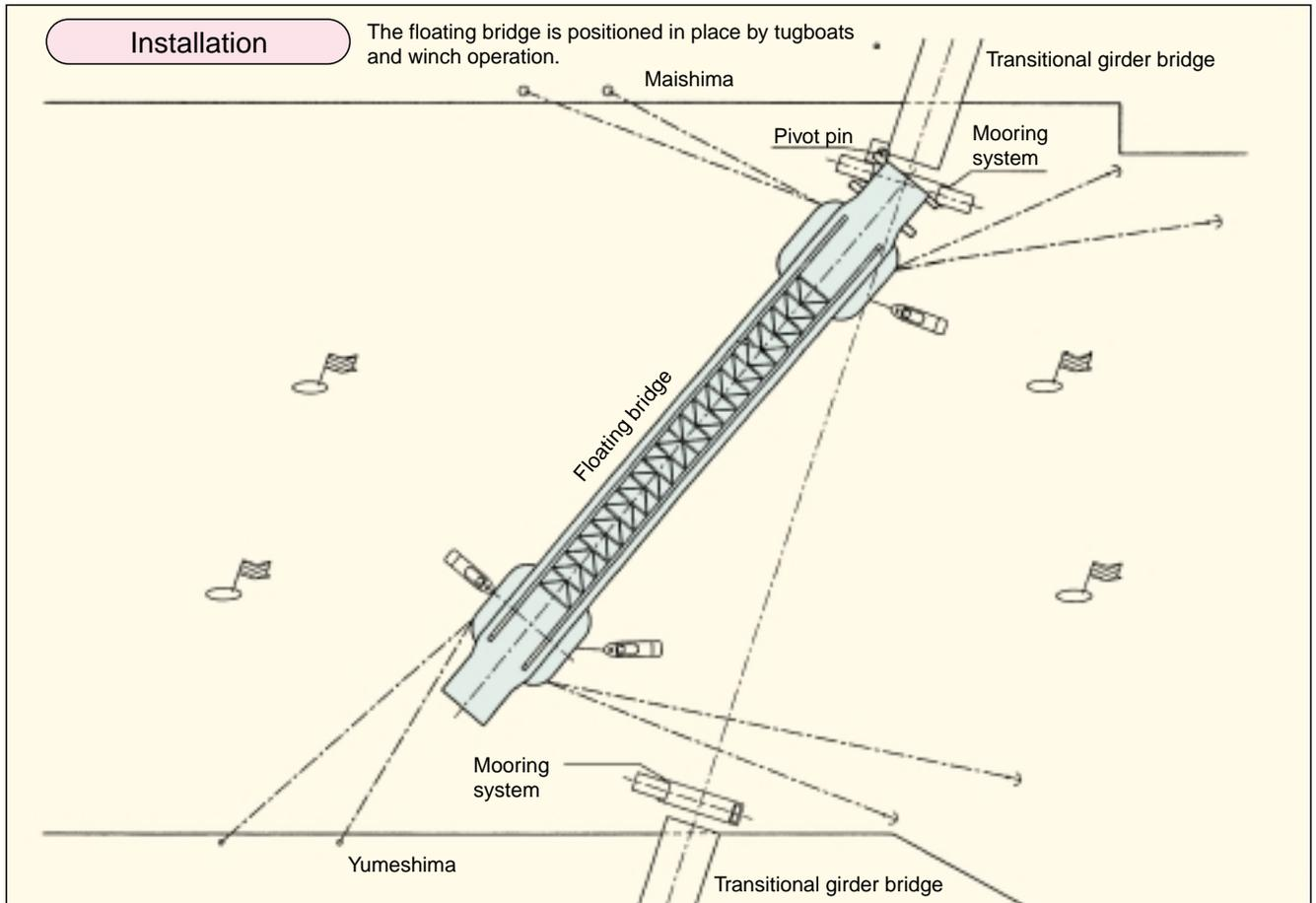
Fig. 16 Pulling out of Dock, Towing & Installation
