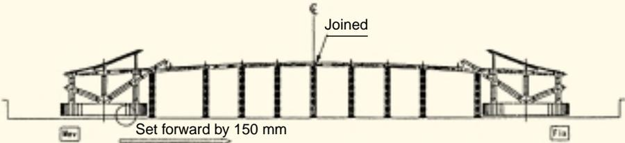
Note) Yumeshima-side axial stopper is unlocked, and Yumeshima-side girder is set forward using hydraulic jack set on stopper, to meet Maishima-side girder.
