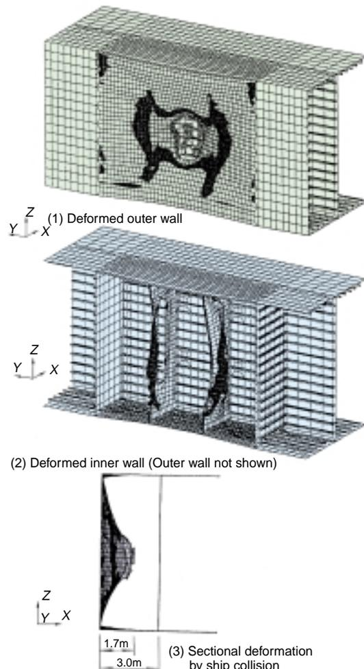
Fig. 14 Results of Ship Collision FEM Analysis
