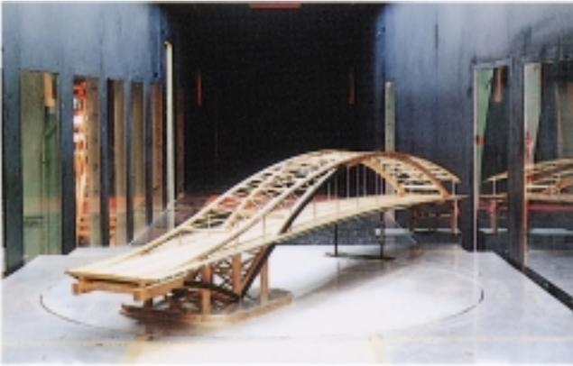
Photo 2 Wind Tunnel Test
