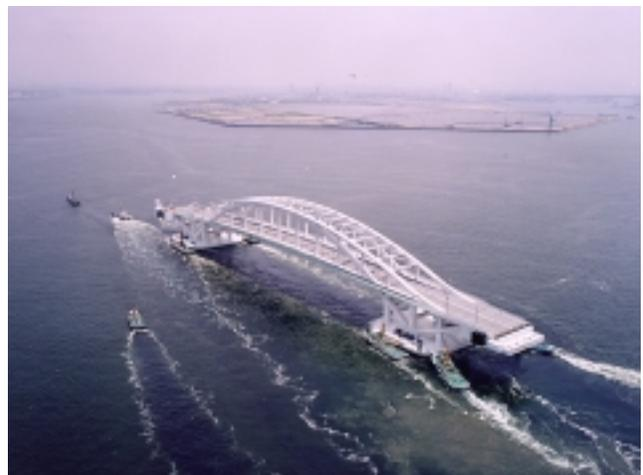
Photo 11 Floating Bridge Is Being Towed
