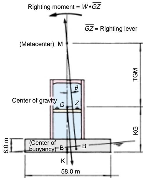
Fig. 4 Centers of Buoyancy and Gravity, and Metacenter
