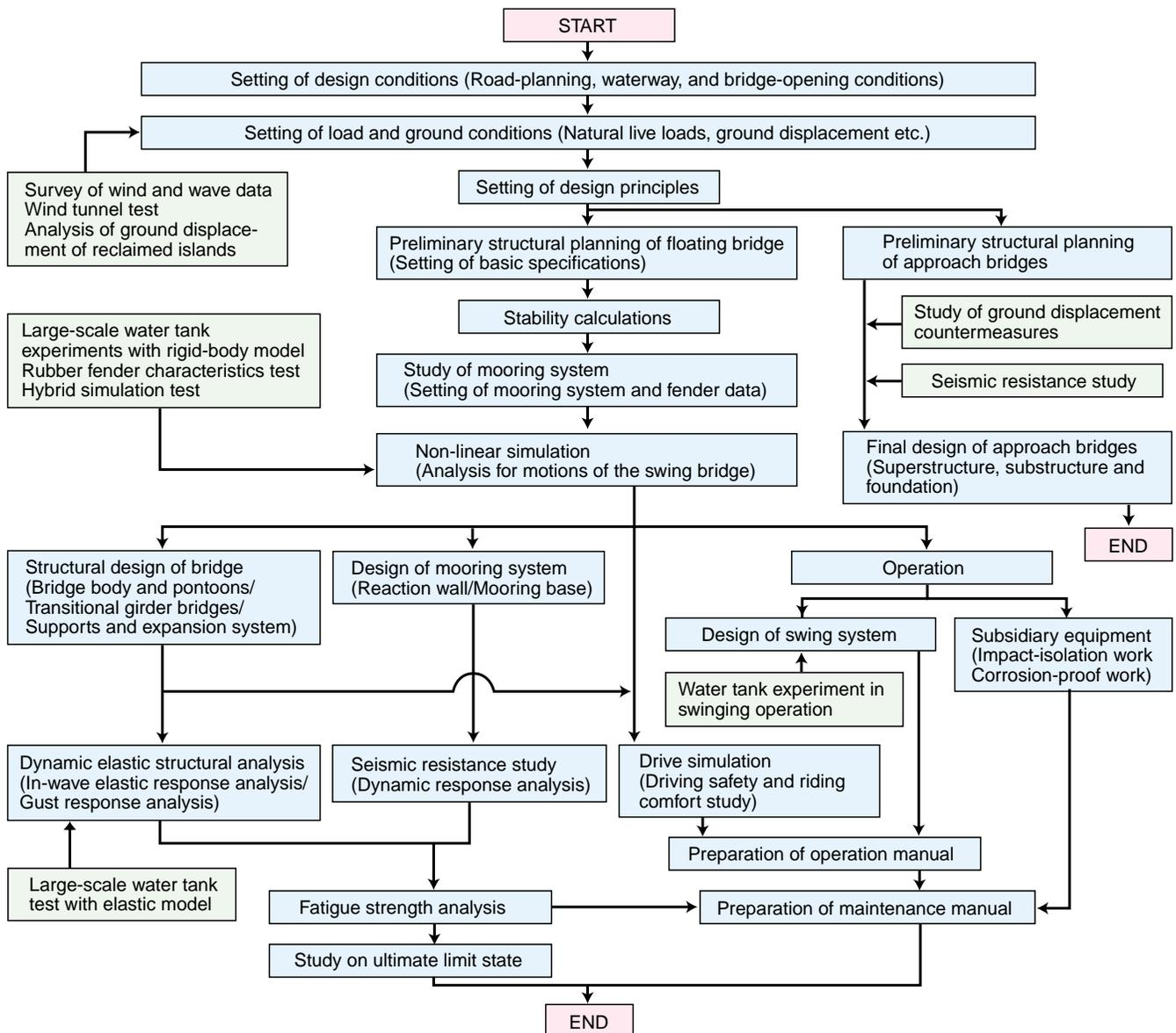
Fig. 3 Flow Chart for Design of Yumemai Bridge
